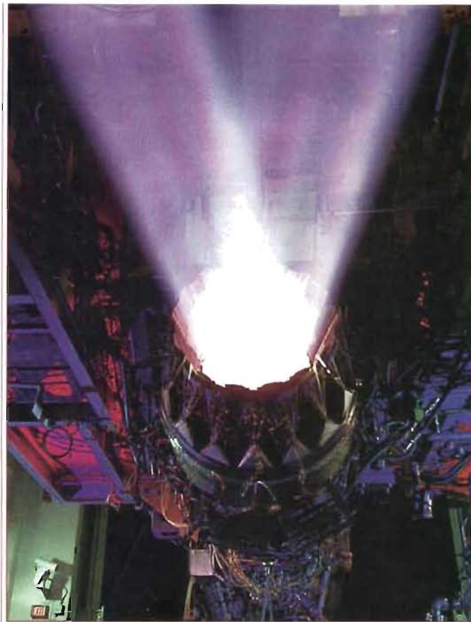
Pratt & Whitneys vektoriserade motor till F-15 ACTIVE (Advanced Control Technology for Integrated Vehicles) vid markprov.
