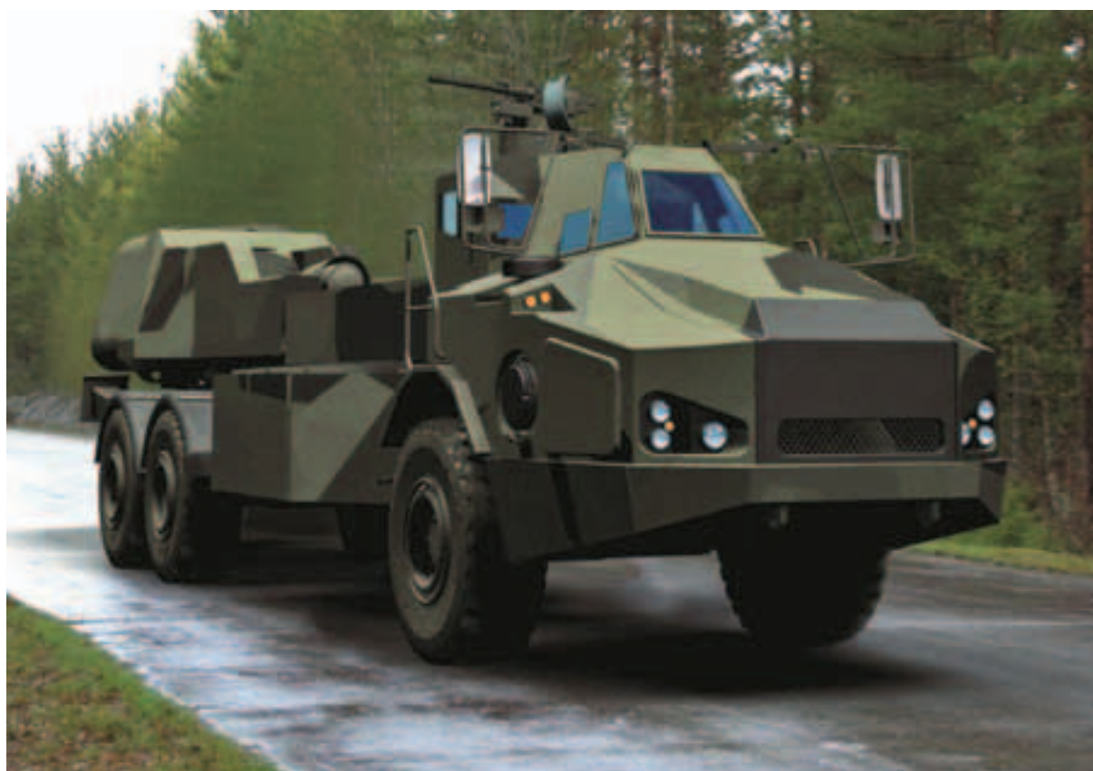
When the Volvo dumper has undergone its full transformation to an Archer unit, the cabin will have been modified beyond recognition, somewhat like the photo above.
