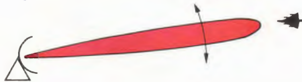
Figure 20. Nodding height finder measurement ("azication" or bringing to bear on target in azimuth from 2D surveillance radar)
