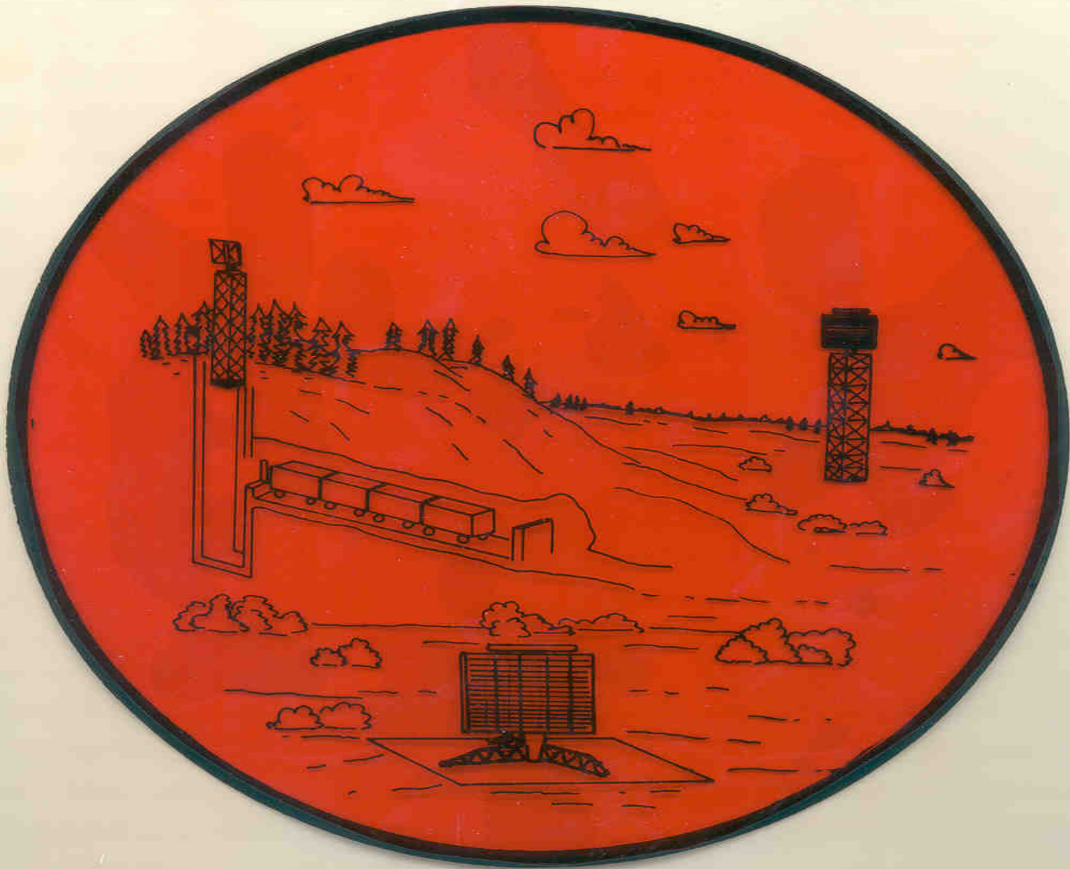
SKETCH OF ITT GILFILLAN 'S' BAND 3D RADAR WITH ANTENNA MOUNTED ON AN ELEVATOR AND RADAR EQUIPMENT IN A TUNNEL
